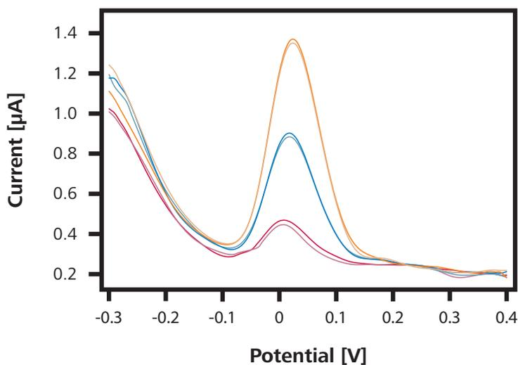
**Figure 7.** Current-voltage curve of an arsenic(III) determination in mineral water with the 946 Portable VA Analyzer with two standard additions of an As(III) standard solution.
