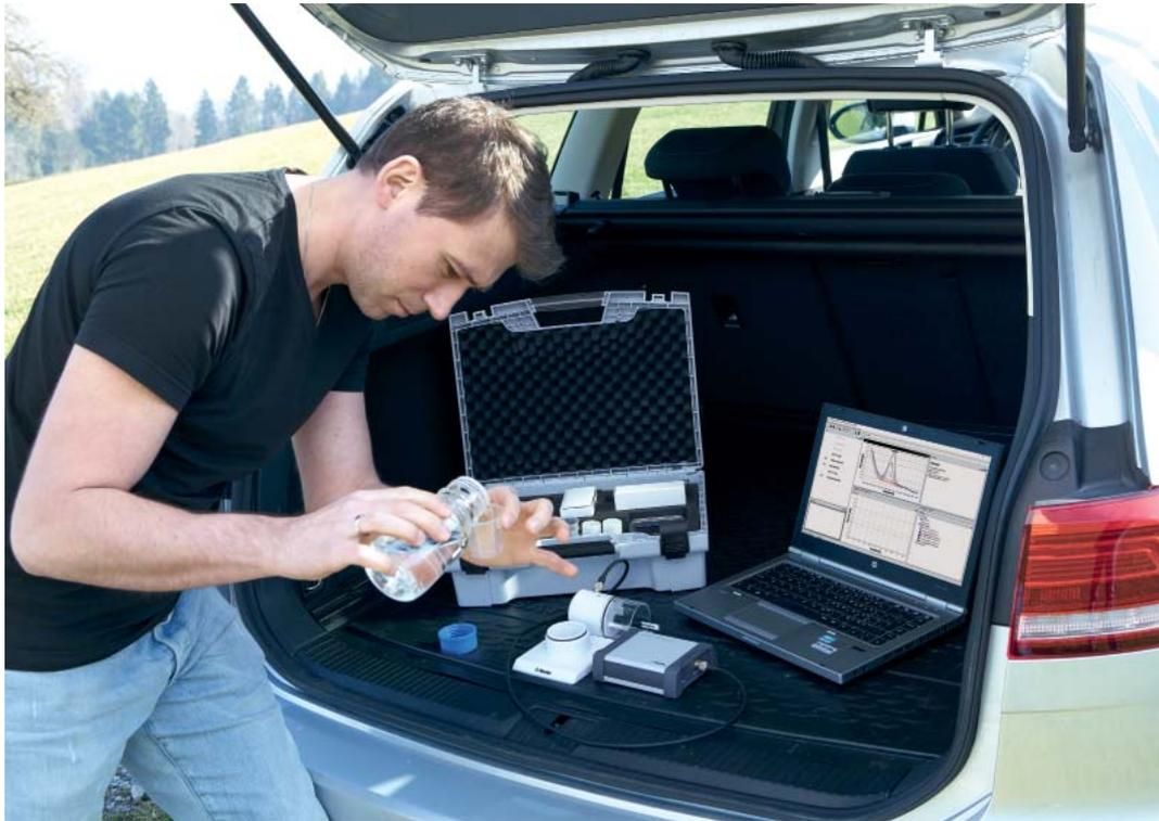
**Figure 6.** The Portable VA Analyzer enables onsite measurements and thus enables, for example, reliable speciation analyses of arsenic. The measuring instrument and the necessary accessories fit in the accompanying handy transport case.
