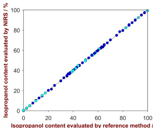
**Fig. 5:** Correlation plot of isopropanol content predicted by NIRS versus reference values. A high correlation is observable. Displayed are the calibration (blue) and the validation data (turquoise).
