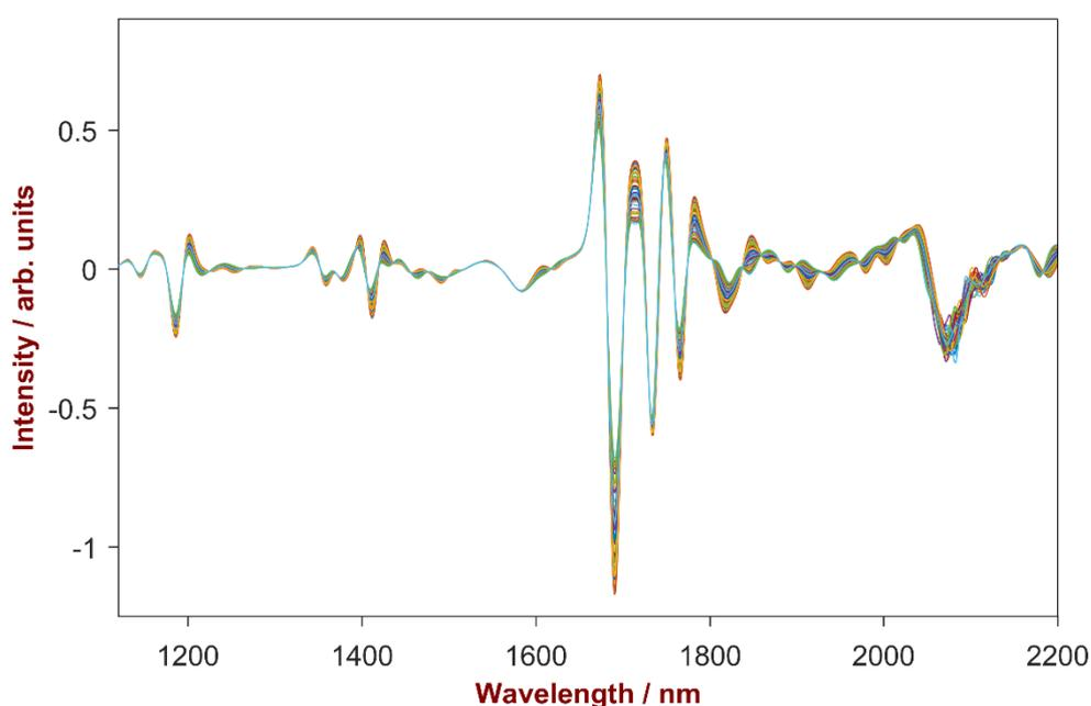
This Application Note describes a fast, nondestructive, and reliable method for the determination of the chemical composition of alcohol mixtures exemplified by ethanol/isopropanol mixtures. With visible near infrared spectroscopy (VIS-NIRS), results are available in real-time, thus making NIRS highly suited for fast quality control.
