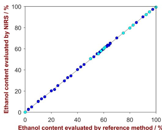
**Fig. 4:** Correlation plot of ethanol content predicted by NIRS versus reference values. A high correlation is observable. Displayed are the calibration (blue) and the validation data (turquoise).
