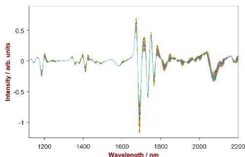
Fig. 3: 2<sup>nd</sup> derivative spectra of 44 ethanol/isopropanol mixtures in the region of 1100–2200 nm.
