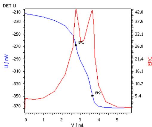
Fig. 1: Determination of  $\text{Ca}^{2+}$  (109.8 mg/L) and  $\text{Mg}^{2+}$  (21.89 mg/L) in tap water from Herisau using a combined Ca ISE.
