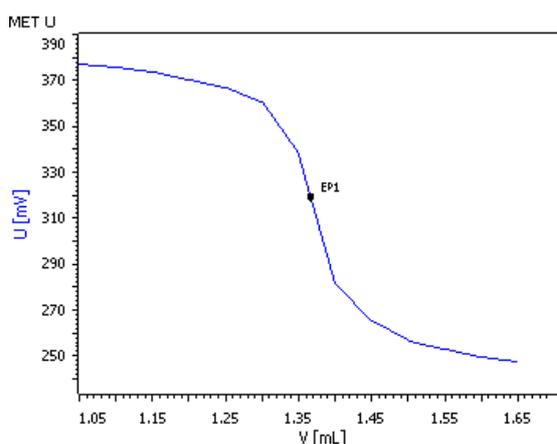
Fig. 3: Determination of the Ca hardness
