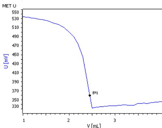
Fig. 2: Determination of the total hardness.
