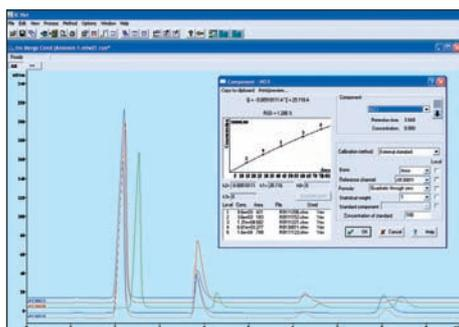
**Fig. 9:** This illustration shows the IC Net interface with ion chromatograms of cationic standards used for a calibration. If problems occur, the IC Net software is ideal for troubleshooting.
