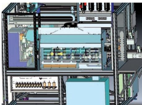
**Fig. 5:** As the transport robot is mounted above the working area, even Erlenmeyer flasks under the fume hood (center of illustration) can easily be accessed.
