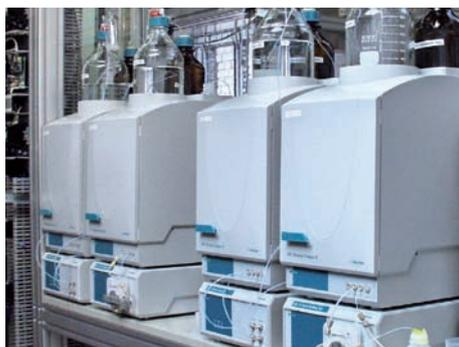
**Fig. 2:** The twin systems, each consisting of two 861 Advanced Compact ICs for the analysis of anions and cations, respectively.
