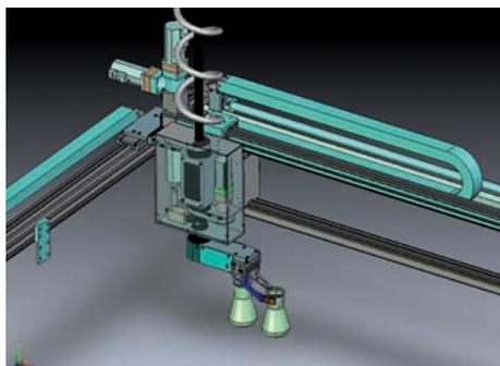
**Fig. 4:** The Nucomat robotic system for transporting samples and containers. The illustration shows details of the robot head with the gripper arm mounted eccentrically on the spindle axis.
