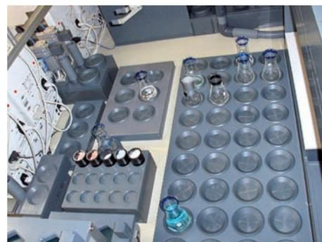
**Fig. 6:** View of the rear panels of the ion chromatographs and the labware of the Wetchem system (mainly wide-neck Erlenmeyer flasks) that are necessary for fully automatic sample preparation.
