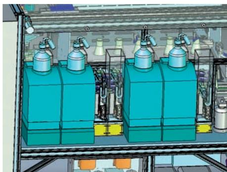
**Fig. 3:** Computer image of the module with the Metrohm ion chromatographs.
