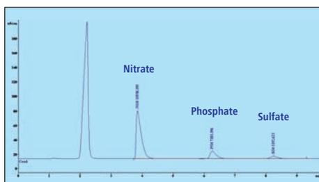
**Fig. 7:** This illustration shows a chromatogram obtained with a fertilizer sample by ion chromatography, in which the nitrate, phosphate and sulfate anions are determined.
