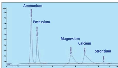
**Fig. 8:** Cations such as ammonium, potassium, magnesium, calcium and strontium can also be determined in the fertilizer sample by ion chromatography.
