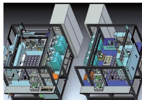
**Fig. 1:** One of Nucomat's product lines is the automated «Wetchem system» for the analysis of liquid chemicals. System characteristics can be described briefly as «untreated sample in, validated result out», as well as the possibility of carrying out several analysis methods.
