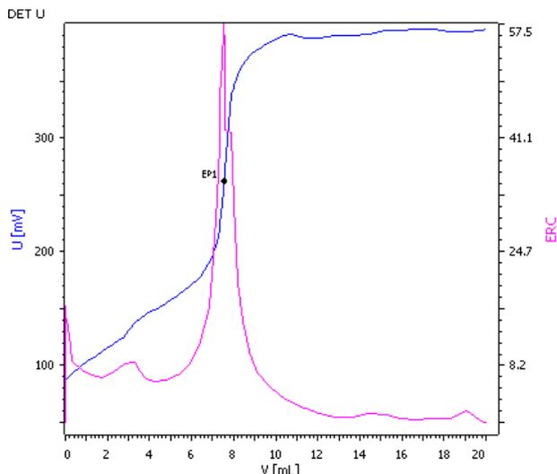
Fig. 3: Determination of the Isocyanate value (blue = titration curve, pink = ERC)
