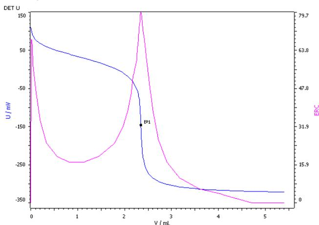
Fig. 1: Determination of the acid value (blue = titration curve, pink = ERC)
