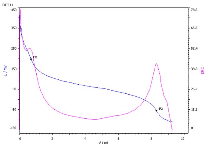
Fig. 2: Determination of the hydroxyl value (blue = titration curve, pink = ERC)
