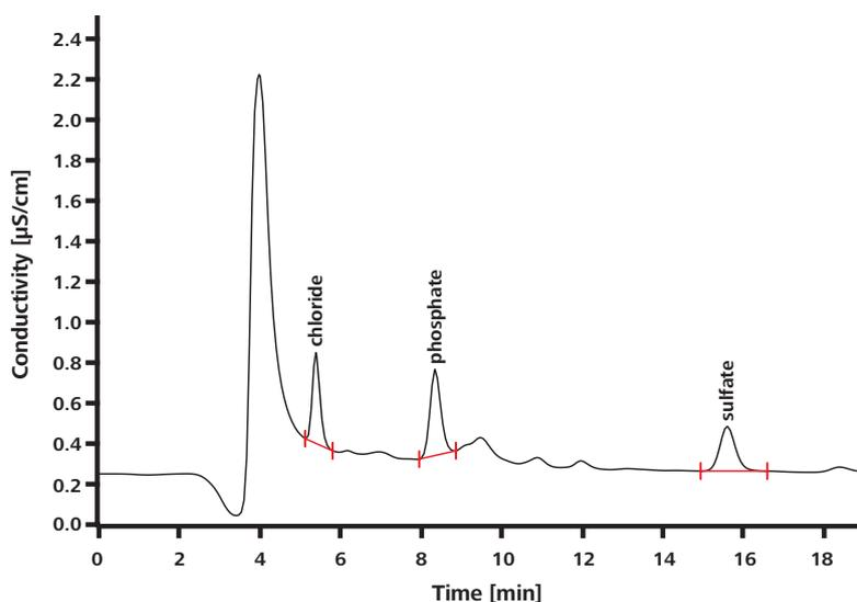
**Figure 4.** Artificial sample from the water-steam circuit of a supercritically operated reactor, with 1 µg/L chloride, 3 µg/L phosphate, and 1 µg/L sulfate added to it; column: Metrosep A Supp 10 - 100/2.0; eluent: 5 mmol/L Na<sub>2</sub>CO<sub>3</sub>, 5 mmol/L NaHCO<sub>3</sub>, 0.25 mL/min; column temperature: 45 °C; preconcentration volume: 4,000 µL
