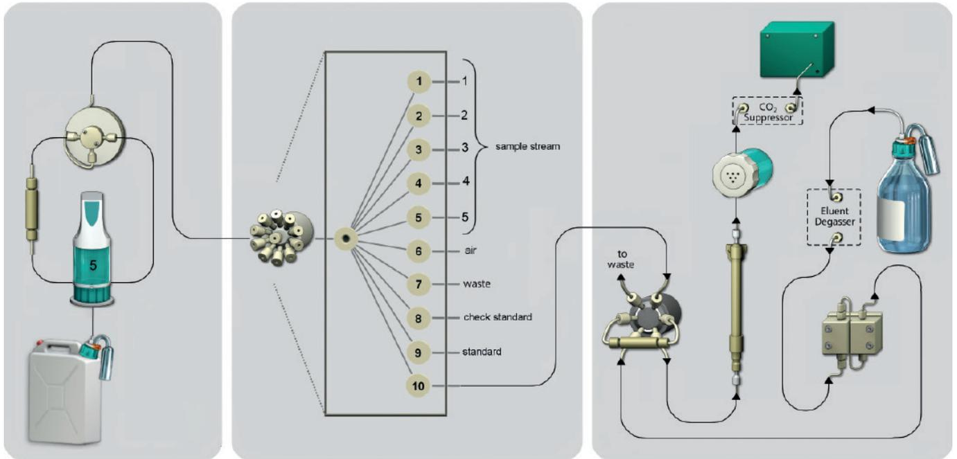
**Figure 3.** Diagram of the Metrohm IC system for online determination of chloride and sulfate traces in the water-steam circuit. It is possible to monitor five freely selectable sample streams alternately. The 10-port selector valve provides further connection points for both the calibration standard and the check standard.
