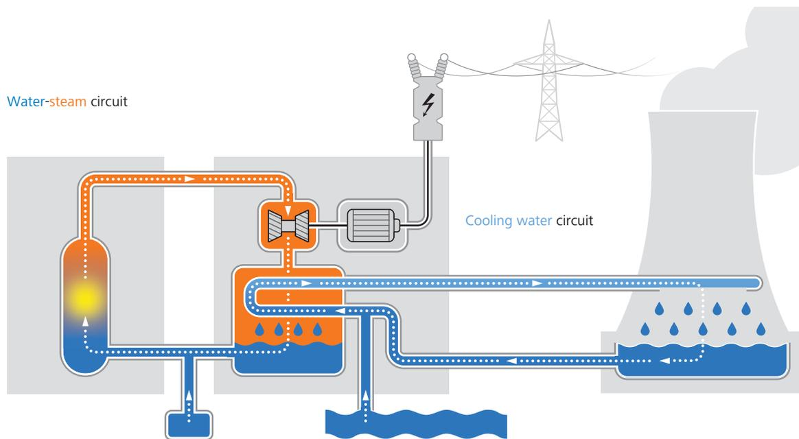
**Figure 1.** The two-circuit system shown here is made up of the water-steam circuit and the cooling water circuit. Water is pumped into the steam generator (on the very left), where it is heated. The steam then migrates through the pipe system to the turbine and drives this, producing electricity. In the condenser, the steam condenses by emitting heat energy to the cooling water. Following this, the water is fed back into the steam generator and the process begins again.
