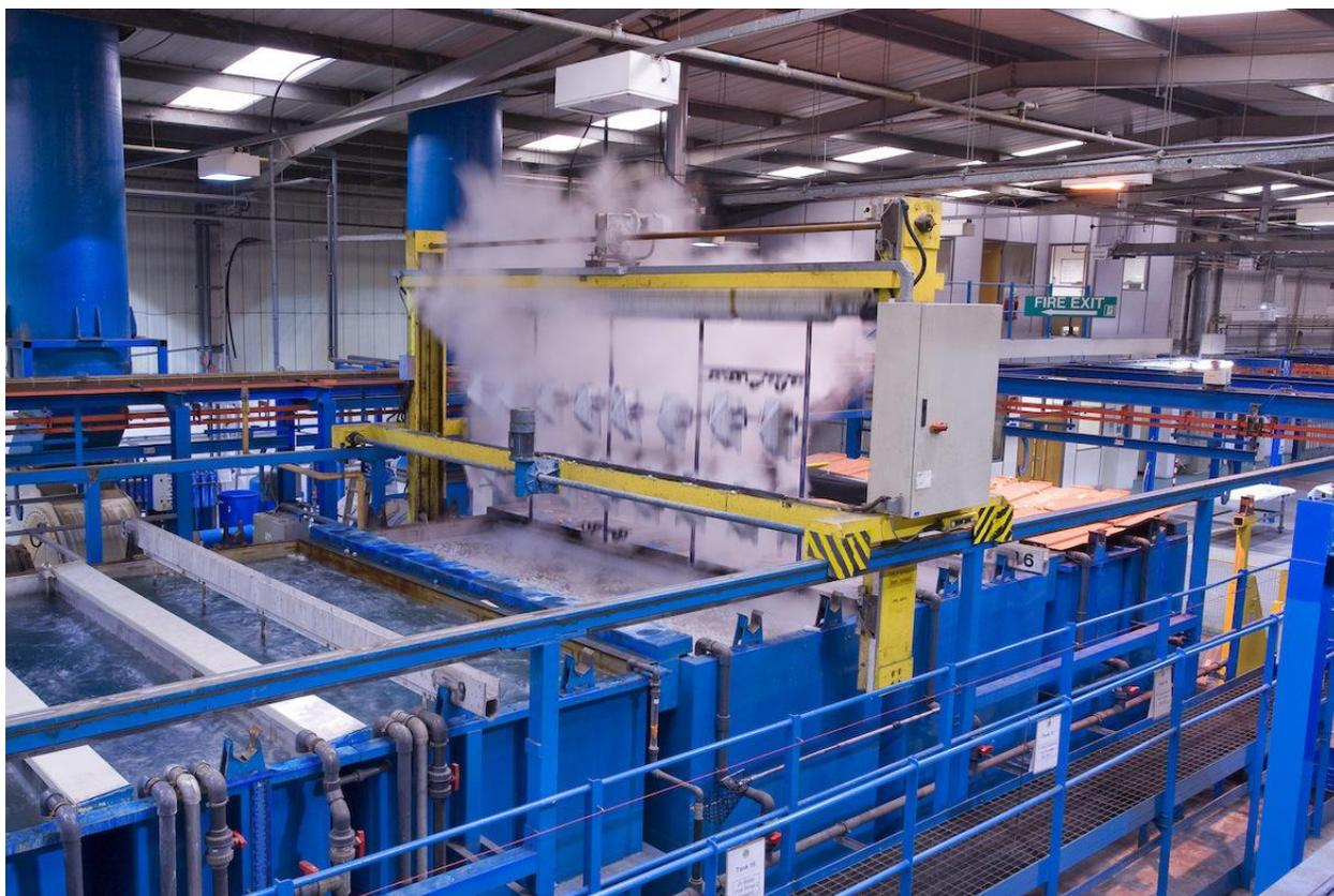
**Application:** On-Line monitoring of the alkaline, acid and aluminium by titration with Process Analyzers ADI 2045TI and ADI 2016 depending on single or multi parameter needs.
