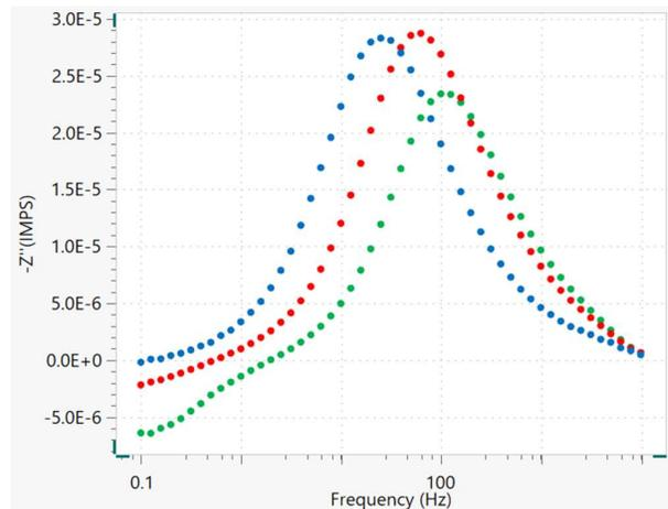
Figure 6 – Imaginary component  $-Z''(IMPS)$  of the IMPS transfer function plotted versus the frequency at 5 mW/cm<sup>2</sup> (blue dots), 10 mW/cm<sup>2</sup> (red dots), and 50 mW/cm<sup>2</sup> (green dots).
