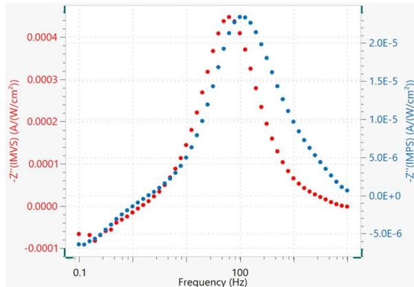
Figure 7 – Comparison of the  $-Z''$  versus frequency plots for IMPS (blue dots) and IMVS data (red dots), obtained at  $50 \text{ mW/cm}^2$
