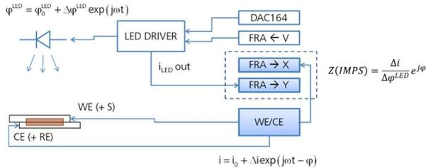
Figure 4 – Overview of the experimental setup of the IMPS measurements
