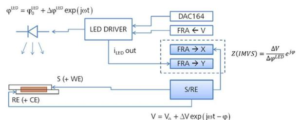
Figure 1 – Overview of the experimental setup for the IMVS measurements.
