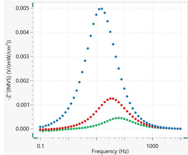
Figure 3 – Imaginary component  $-Z''(IMVS)$  of the IMVS transfer function plotted versus the frequency at 5 mW/cm<sup>2</sup> (blue dots), 10 mW/cm<sup>2</sup> (red dots), and 50 mW/cm<sup>2</sup> (green dots).
