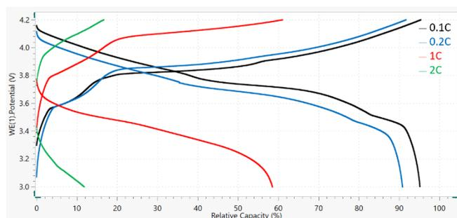
Figure 2 – Potential vs. relative capacity plot, at different C-rates
