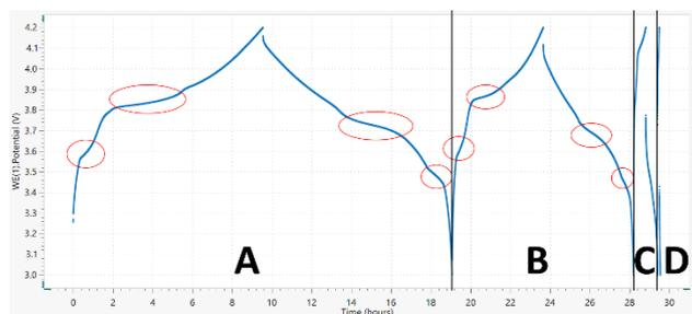
Figure 1 – Potential vs. time at different C-rates. Section A, 0.1C; Section B, 0.2C; Section C, 1C; Section D, 2C. The red circles highlight the plateaus at 0.1C and 0.2C.
