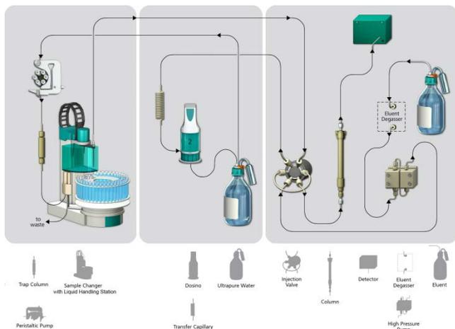
Prepare and degas an eluent suitable for the column you want to use (see column manual). For Metrosep C 4 - 150/4.0 a solution of 1.7 mmol/L HNO<sub>3</sub> / 0.7 mmol/L dipicolinic acid (DPA, 2,6-Pyridinedicarboxylic acid) is adequate.
