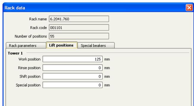
In order to configure the settings of the Liquid Handling Station, two external needle positions have to be defined for the tower of the Sample Processor in the window configuration. At the “external position 1” the needle should be in the inner compartment of the rinsing part which corresponds to an angle of approximately 106° and a work position of 125 mm. The exact angle depends on your installation. In this position, the needle is rinsed from the in- and outside.
