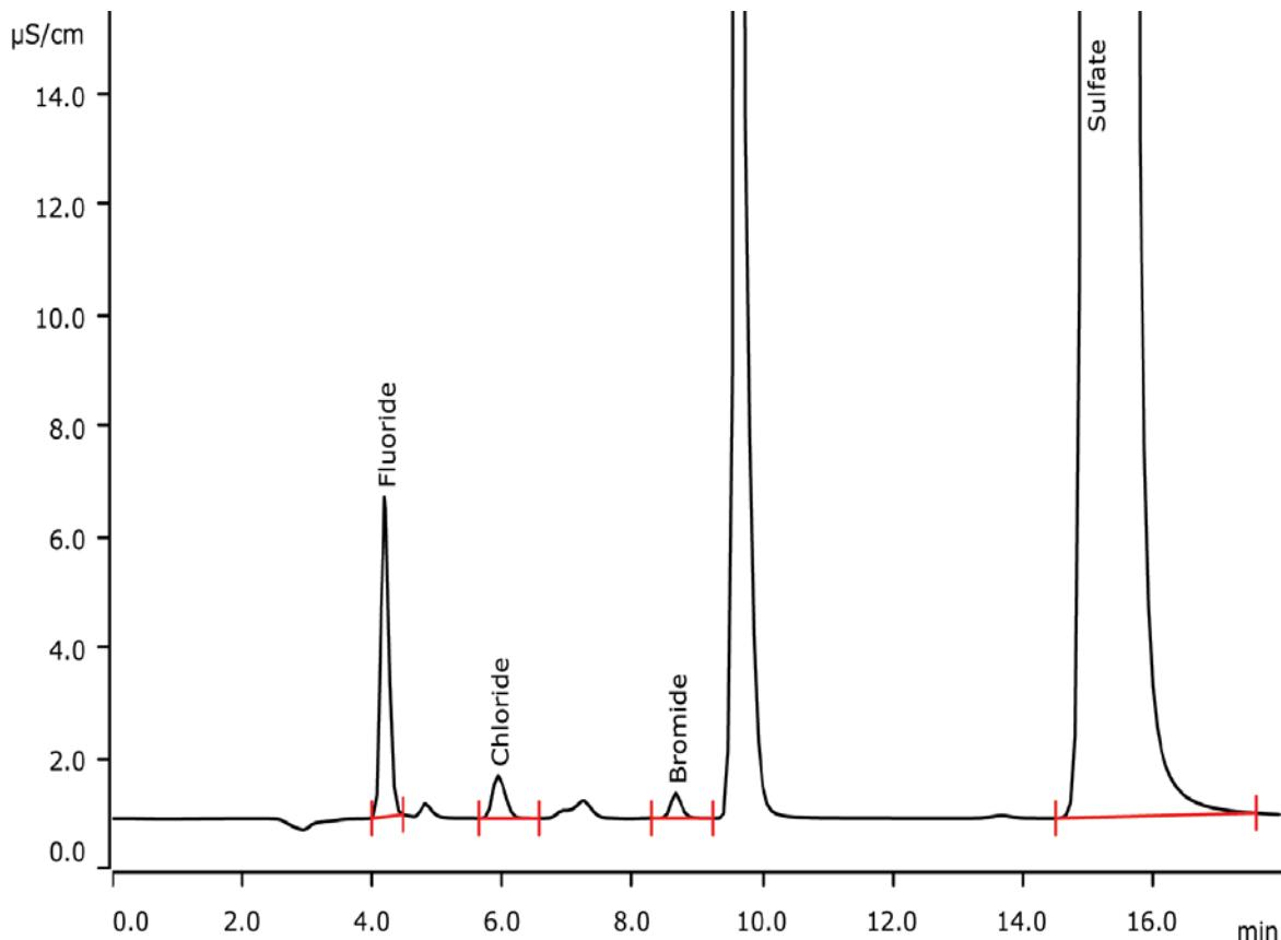
Combustion of coal releases halogens into the atmosphere. In coal, fluorine and chlorine are of natural origin, whereas bromine is often added to reduce mercury emissions. Here, the results of Combustion IC for three coal samples with varying bromide levels are presented.
