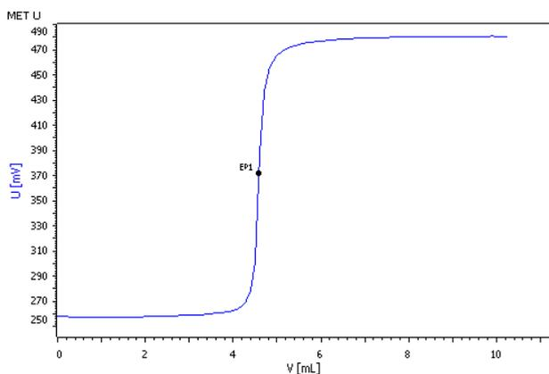
Fig. 2: Photometric Kjeldahl nitrogen determination in MET modus
