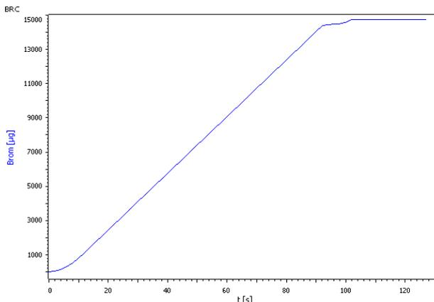
Fig. 4: Coulometric nitrogen determination in BRC modus
