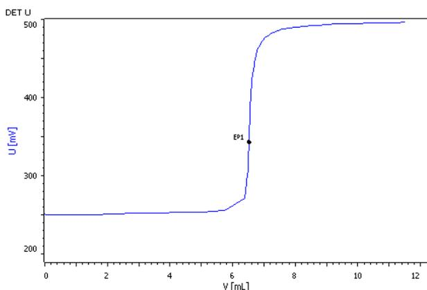
Fig. 3: Photometric Kjeldahl nitrogen determination in DET modus
