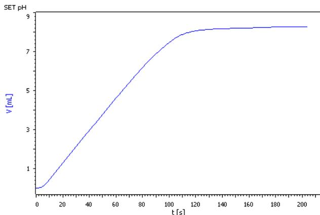
Fig. 1: Potentiometric Kjeldahl nitrogen determination in SET modus
