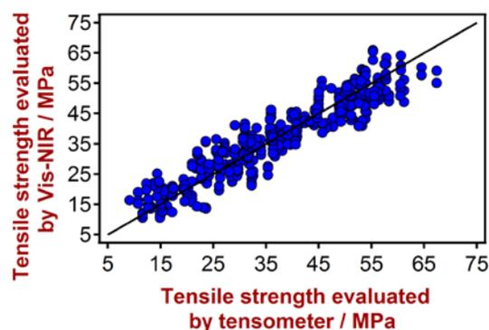
**Fig. 7:** Correlation plot of reference values from tensometer versus predicted values from Vis-NIR. The tensile strength varies between 8 – 68 MPa.
