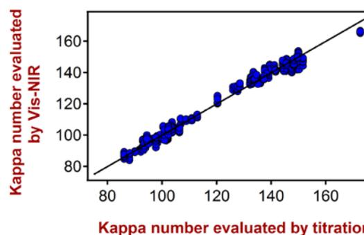
**Fig. 3:** Correlation plot of reference values from titration versus predicted values from Vis-NIR. The Kappa number varies between 74.6 – 174.6 mg.
