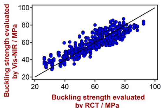
**Fig. 6:** Correlation plot of reference values from Ring Crush Test (RCT) versus predicted values from Vis-NIR. The buckling strength varies between 26.3 – 92.4 MPa.
