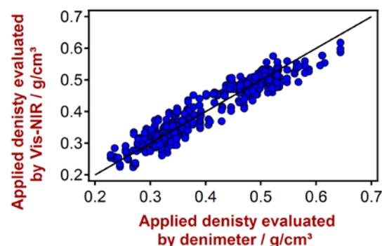
**Fig. 8:** Correlation plot of reference values from densimeter versus predicted values from Vis-NIR. The applied density values vary between 0.2280 – 0.6437 g / cm<sup>3</sup>.
