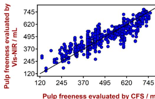
**Fig. 4:** Correlation plot of reference values from Canadian Standard Freeness (CSF) versus predicted values from Vis-NIR. The pulp freeness varies between 130 - 740 mL.
