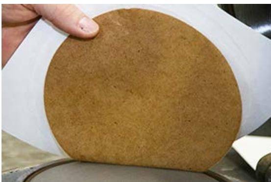
**Fig. 1:** Standard hand sheets for testing of pulp quality
