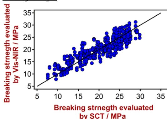
**Fig. 5:** Correlation plot of reference values from Short Span Comprehensive Strength Test (SCT) versus predicted values from Vis-NIR. The breaking strength varies between 7.6 – 29.8 MPa
