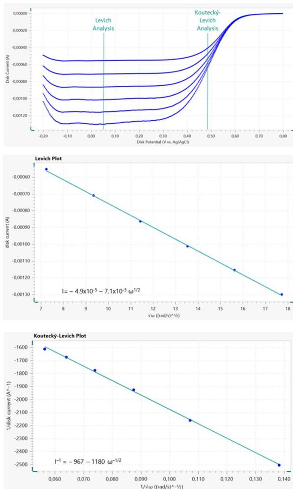
Figure 2 - Linear sweep voltammetry profiles (top) from the disk electrode at various rotation rates; the potential value for the Levich and Koutecký-Levich analyses are indicated. Levich (middle) and Koutecký-Levich (bottom) plots.
