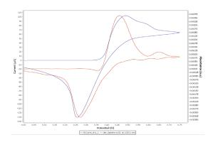
Workspace allows to combine in the same window electrochemical and optical data (cyclic voltammogram in blue, derivative voltabsorptogram in red).
