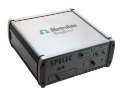
Metrohm DropSens provides you with one instrument combining Light source (VIS-NIR: 360-2500 nm Tungsten halogen), a Spectrometer (Wavelength range: 900-2200 nm) and a Bipotentiostat/Galvanostat ( $\pm$  4 V DC potential range,  $\pm$  40 mA maximum measurable current).
