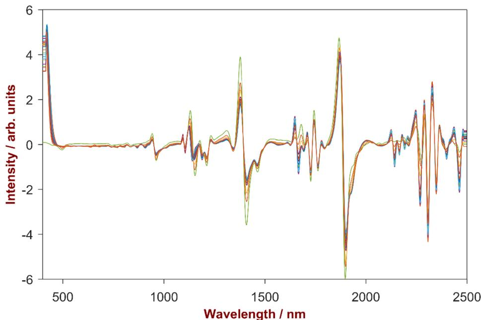
This Application Note shows that visible near-infrared spectroscopy (Vis-NIRS) can determine the sun protection factor (SPF) of sunscreen products. Thanks to measurement durations of less than 30 seconds, NIR spectroscopy is ideally suited for rapid quality control.
