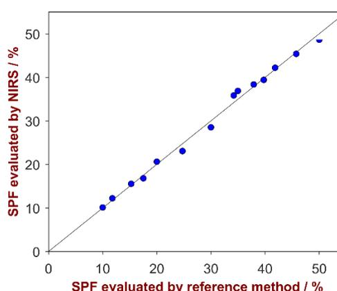
Fig. 5: Correlation plot of SPF predicted by Vis-NIRS versus the reference values. A high correlation is observable.
