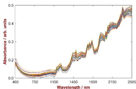
**Fig. 2:** Vis-NIR spectra of Cefixime tablets over the full wavelength range.
