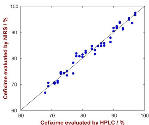
**Fig. 4:** Correlation plot of the Cefixime content predicted by NIRS versus the reference values.
