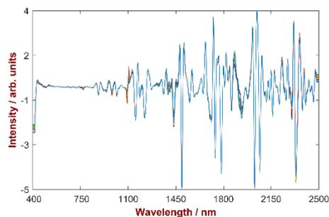
**Fig. 3:** Spectra pretreated with 2<sup>nd</sup> derivative and SNV over the full wavelength range.
