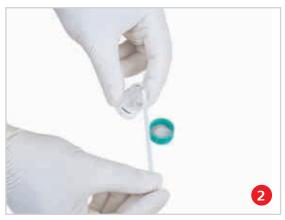
Using the provided spatula, transfer a small amount of sample to the vial, 2–3 mg is sufficient, but more sample will provide a stronger signal.
