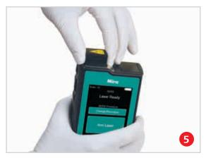
Mount the SERS attachment onto Mira DS and turn on the instrument.
