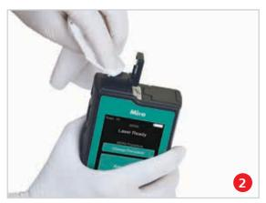
Wipe down interior surfaces using a kimwipe or swab, ethanol or isopropanol may be used. Cleaning is intended to remove residue from previous substrates, rather than polishing the window.
