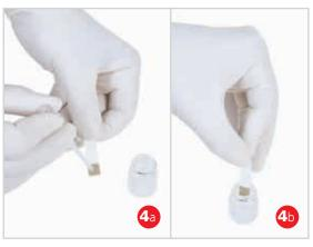
Apply sample to the P-SERS test strip using one of two methods:
