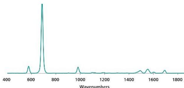
Figure 2. Standard Ag P-SERS reference spectrum of melamine.
