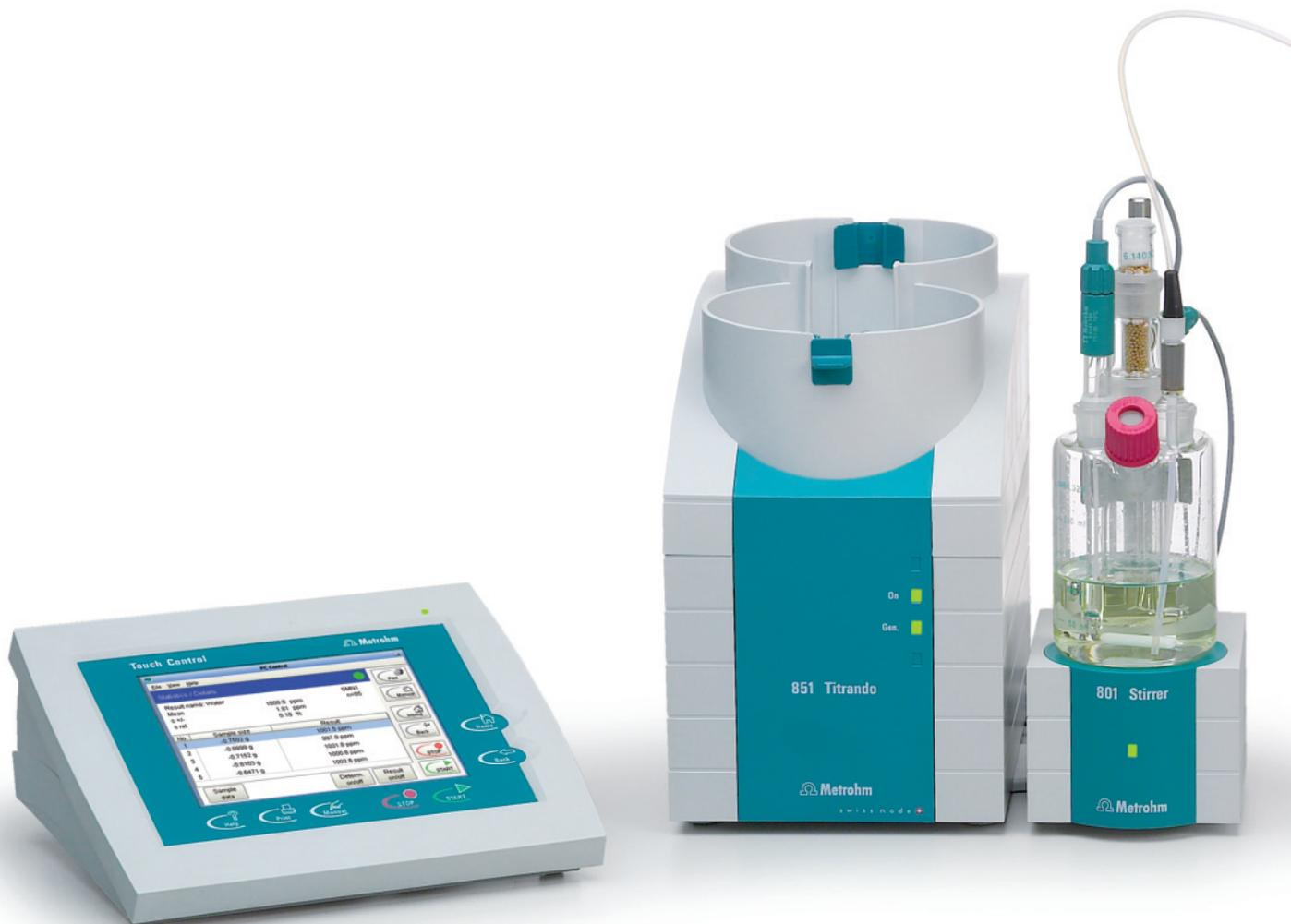
851 Titrande with KF Evaporator and Touch Control. The perfect instrumentation for water determination in liquid samples that can neither be analyzed directly nor by the oven method.
