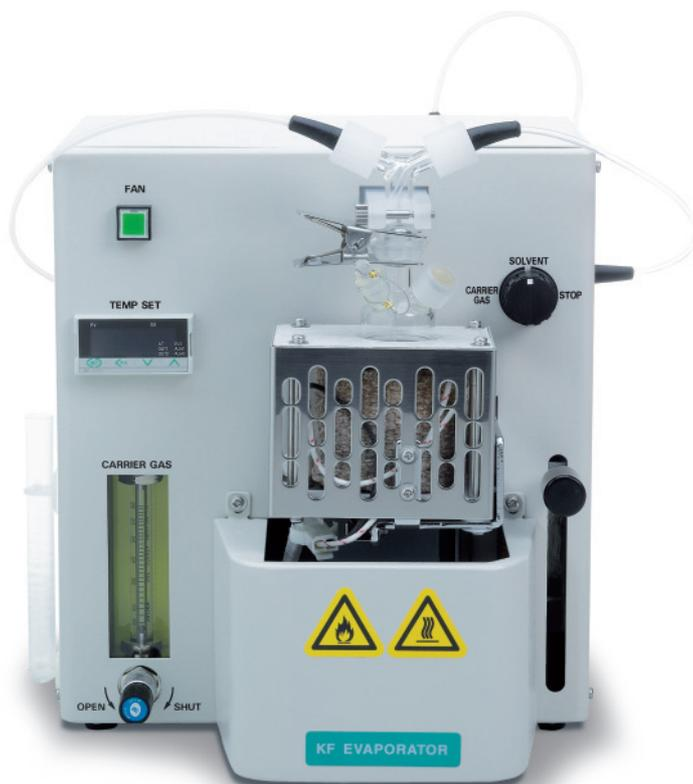
The oven is raised with a finger and the sample heated. Secondary reactions hardly occur, as the sample itself does not reach the titration cell.
