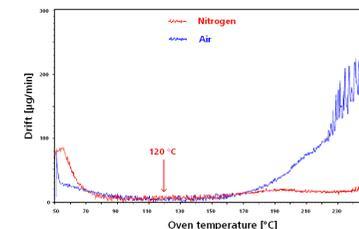
Based on the knowledge obtained from the heating curve, the following water determinations were performed at an oven temperature of 120 °C.
