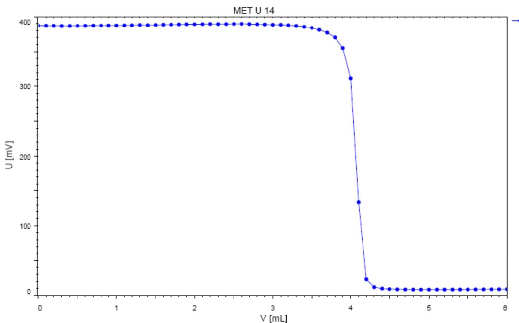
This Application Note describes the photometric determination of aluminum in cement by titration of the digested sample using the Optrode (574 nm). After titration of the dissolved aluminum with EDTA, the EDTA excess is back-titrated with zinc sulfate solution.
